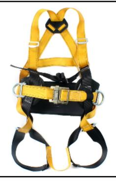
The RGH3 combines the basic fall arrest harness with a comfortable work-positioning belt in one unit. The harness is fitted with a rear dee and two side dee rings mounted to the belt and can be used similar to the RGH1 (see data sheet). When fitted with a pole/work-positioning belt (RGP1&2), the harness can be used for pole climbing or work-positioning on open structures. In certain circumstances, the side dee's on the RGH3, can be used for work restraint in the horizontal plane.
