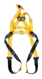
The RGH5 is designed for use as a confined access harness. The front and rear attachment points can be used as standard fall arrest points and the rescue strap can be used for lifting and lowering. When used, the rescue strap keeps the operative in a near vertical position, which is preferred when recovering an unconscious casualty.
